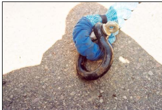
Photo 5. Screw pin shackle (also known as Farm Clevis). (Photo courtesy of County Sheriff's office.)
