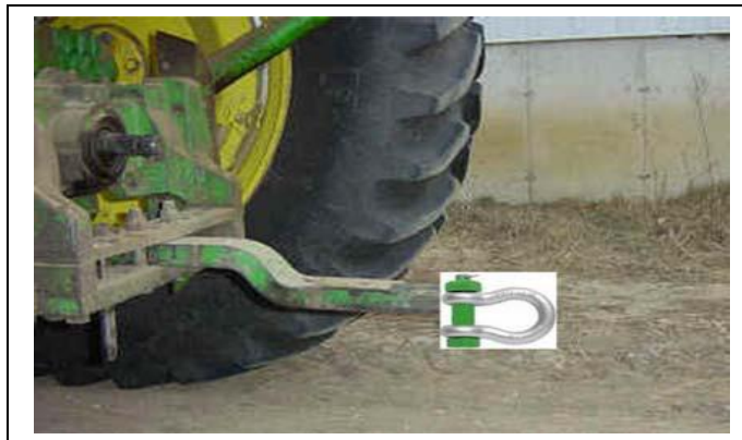
Shackle and tow bar of the tractor shown. The shackles used had a 17 000 lbs working load limit each.
